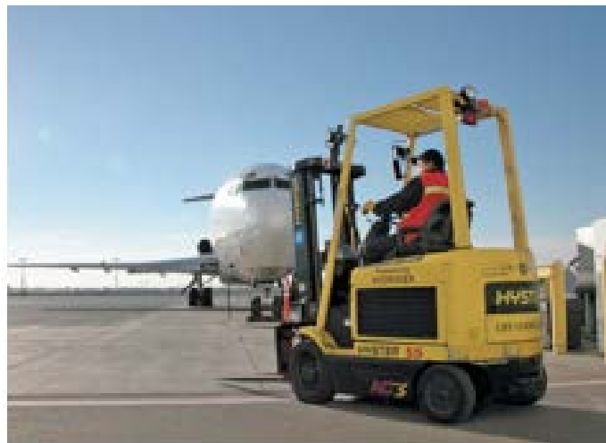
Figure 3. A hydrogen fuel cell forklift in airport service. Photo courtesy of Hydrogenics, NREL 15987
